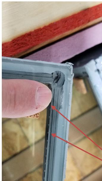
Streaks of black PIB in gray PIB due to incomplete purging of the extruder when color is changed. (Refer to 3.5.1.4)
