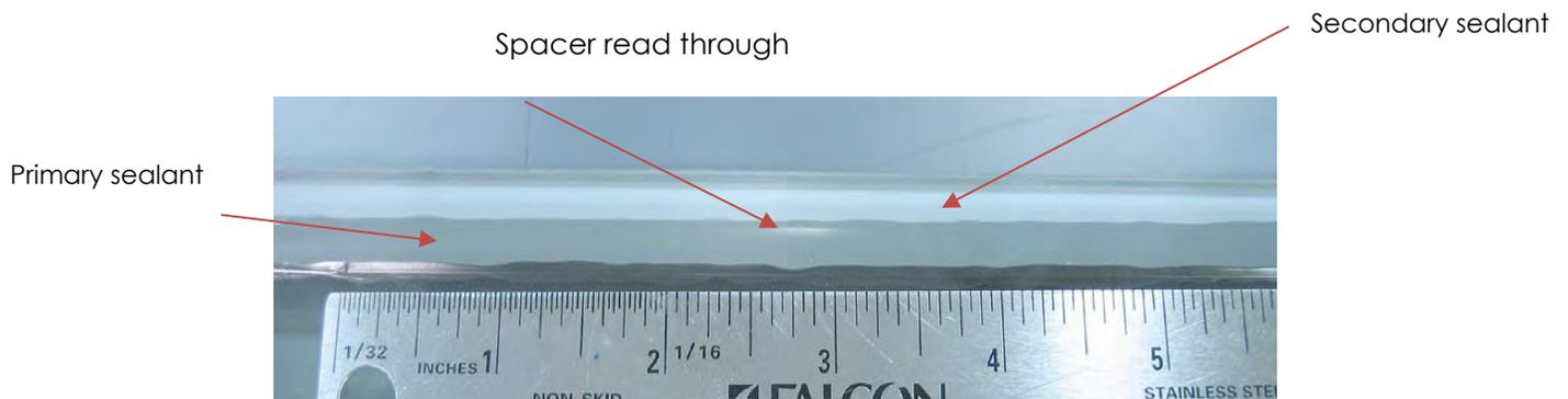
Figure 3.1.1, Spacer Read through
