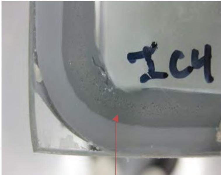
Figure 3.4.2, Bubbles in Sealant
